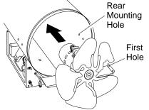
Figure 8 - Fan and Motor Turned Around
